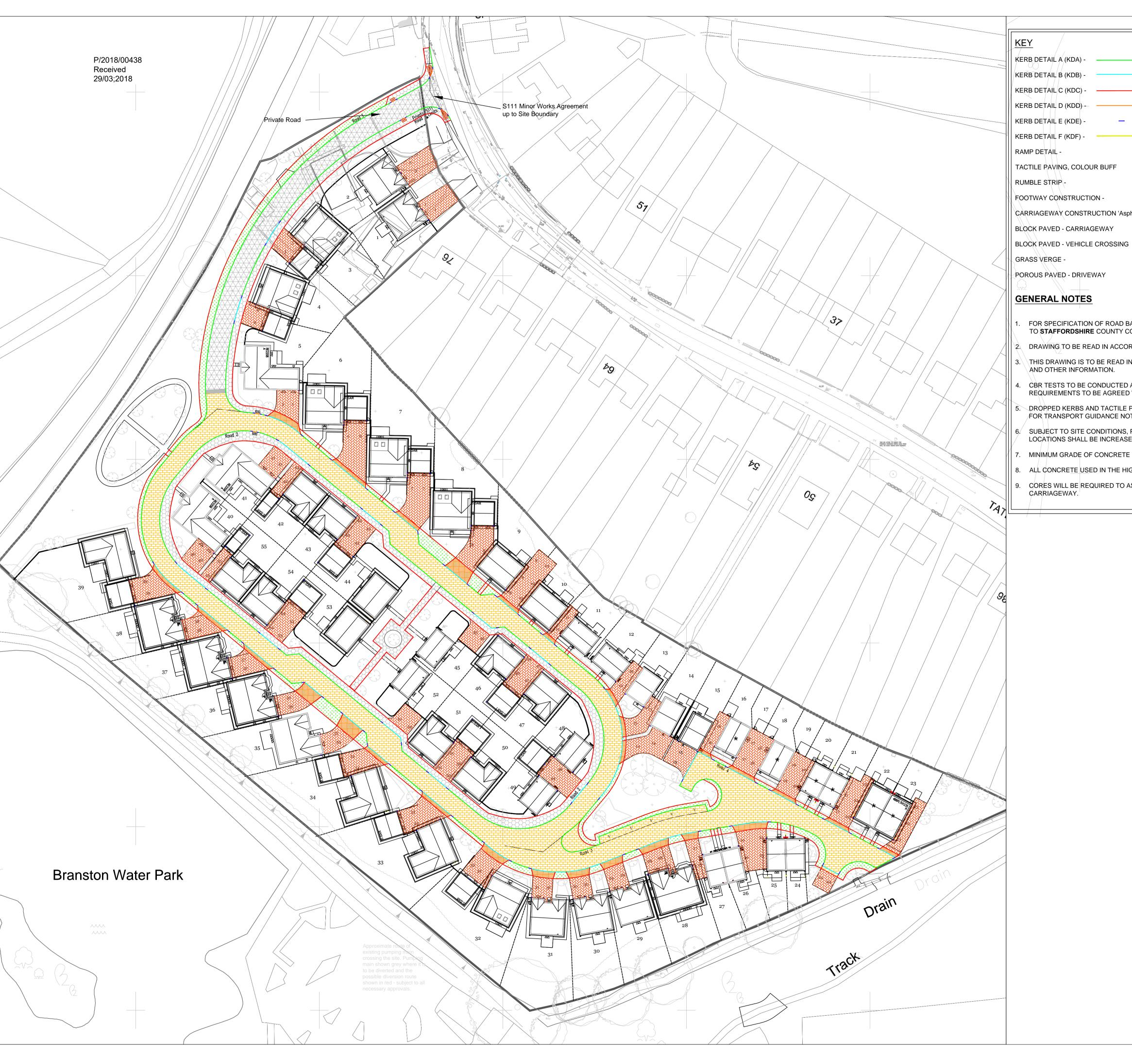
KERB DETAIL A (KDA) -TYPE HB2 (125mm upstand) - DETAIL A KERB DETAIL B (KDB) -TYPE BN (25mm upstand) Drop Kerb - DETAIL B KERB DETAIL C (KDC) - -TYPE EF (0mm upstand) - DETAIL |C TYPE BN (0-6mm upstand) - DETAIL D KERB DETAIL D (KDD) -TRANSITION KERB (TYPE HB to BN) KERB DETAIL E (KDE) -KERB DETAIL F (KDF) -255 X 125 SQUARE CHANNEL KERB LAID FLUSH TACTILE PAVING, COLOUR BUFF FOOTWAY CONSTRUCTION -- To SCC Specification
